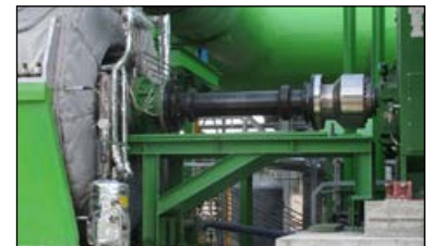
Euroflex Couplings are of all-metal construction and are fully-machined for higher speeds required by turbine-driven gas and liquid process equipment. High performance applications requiring speeds in excess of 20,000 rpm and API 671 compliance can be supplied.
