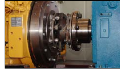
Thomas AMR and CMR Couplings feature cast iron or steel center members engineered specifically for the continuous alternating or vibratory torque loads and slow to medium speeds required for reciprocating applications.
