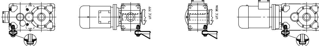
Semi-flexible reaction arrangement, **using disc springs and bracket**
