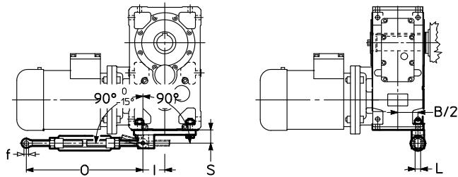
Flexible reaction arrangement using **rubber buffers** (drawings are approximate, but the buffers will be positioned abutting with gear reducer housing). It is possible to install safety devices against accidental overloads.
