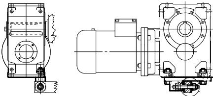
**Rigid torque arm** arrangement for variable distance anchorage (ch. 4).
