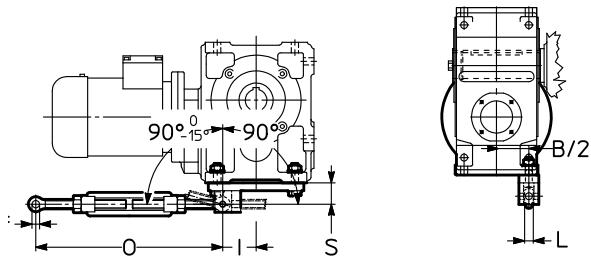
Reaction arrangement see above (ch. 4), but **flexible**; safety devices may be installed to prevent accidental overloads
