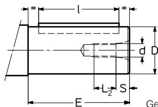
Gear reducer shaft
