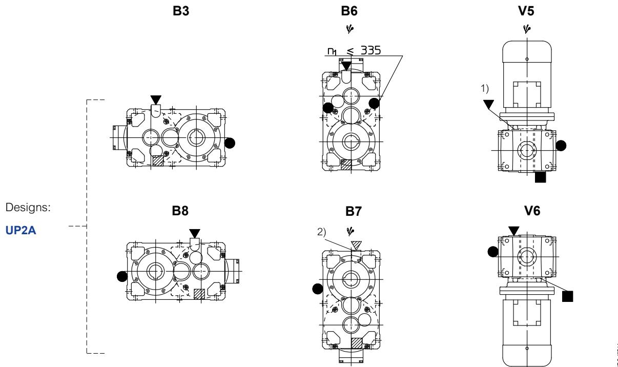
1) Oil filler plug possible even on low speed shaft side.
