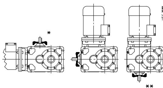
\* Fan position is not possible for train of gears C2I.
