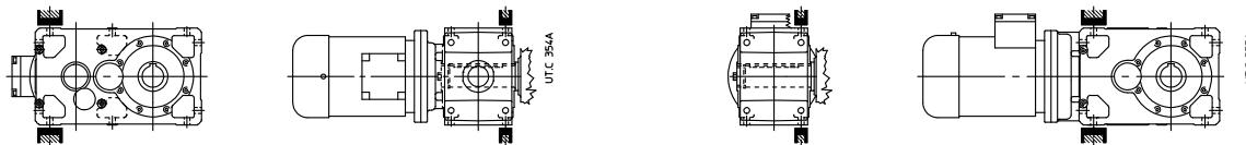
For the majority of normal cases, where weight force  $G$  is parallel or orthogonal to reaction  $R_R$  as illustrated in the drawings, reactions are calculated thus (verify the worst condition) valid for long model too, if applicable:
