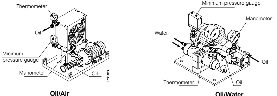
Additional cooling device in the event that the other forced cooling systems are not sufficient for the dissipation of thermal power produced by gear reducer during operation (see ch. 3.3).
