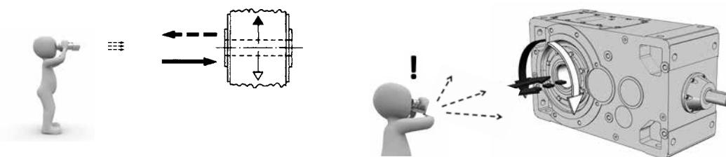
Radial loads generated on the shaft end by a drive connecting gearmotor and machine must be less than or equal to those given in the following pages.
