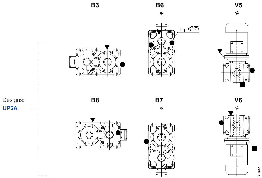
⚠ Possible high oil splash: for the corrective factor  $f_3$  of nominal thermal power  $P_{t_N}$  see ch. 3.
