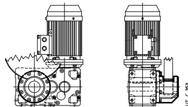
Semi-flexible and economic **reaction arrangement, using disc springs**. Safety devices may be installed to prevent accidental overloads.
