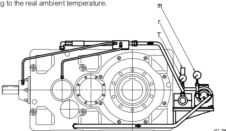
**Sketch of forced lubrication with cooling unit:** the exact position of cooling unit depends on the gear reducer size, train of gears, mounting position and available overall dimensions: for this reason, on request, a drawing of the specific solution will be supplied; the pipes will be realized with suction and delivery flexible pipes and with rigid pipes between the distributor and the bearings.
