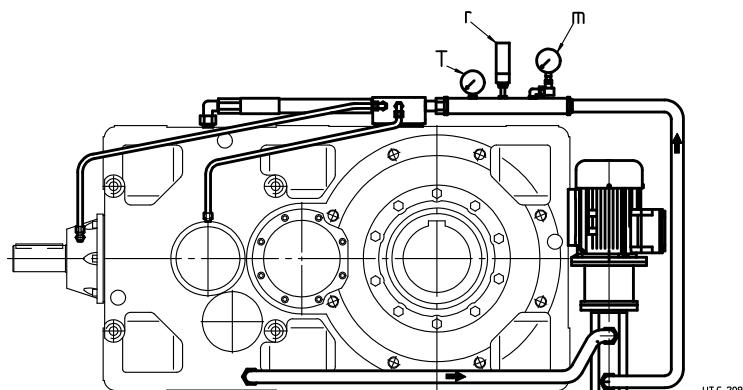
**Sketch of forced lubrication with motor pump:** the exact position of motor pump depends on the gear reducer size, train of gears, mounting position and available overall dimensions: for this reason, on request, a drawing of the specific solution will be supplied; the pipes will be realized with suction and delivery flexible pipes and with rigid pipes between the distributor and the bearings.
