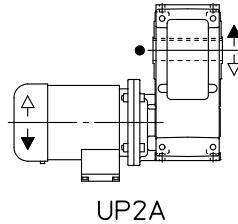
● Position of reference groove (see ch. 3) for radial load verification.
