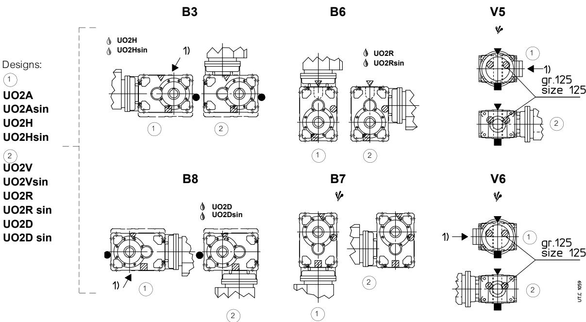
⚠ Possible high oil splash: for the corrective factor  $\frac{P}{P_N}$  of nominal thermal power  $P_N$  see ch. 3.3.
