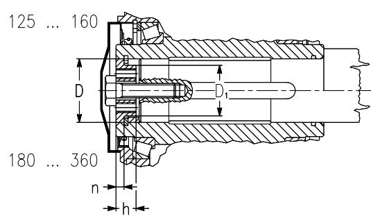
A **washer** for gearmotors installing, removing and gearmotor axial fastening and hollow low speed shaft **protection cap** can be supplied on request.
