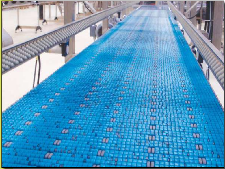
CONVEYOR FOR TRAYS WITH CANS.
