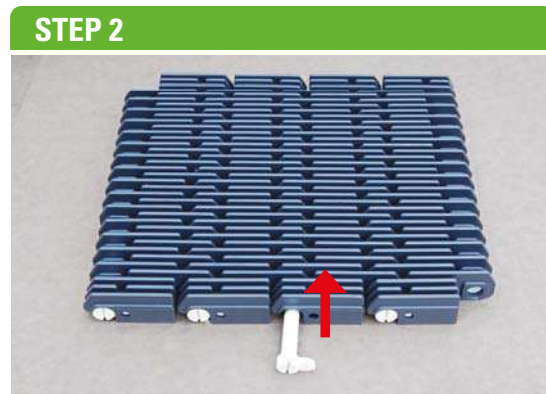
2 - Insert the pin-clip inside the hinge. Push till end position following red arrow direction.
