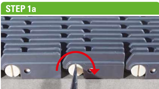
1a - Put the screwdriver in the pin-clip and rotate (clockwise) as pictured above.
