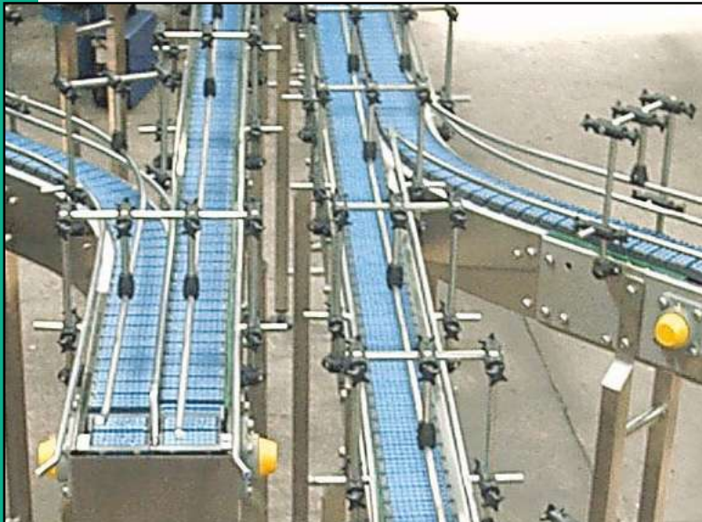
Accumulation system for conical products. The guide on top improves product stability.
